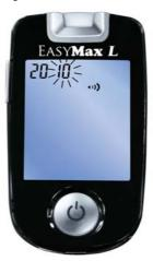
2. Repeat step 2 to 4 in the page 13 to set the year, date, time and sound volume. The flashing field is the one you are currently setting.
