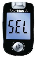
Keep pressing "A" until you see the "SEL". After 2 seconds the meter enters the setting mode automatically.
