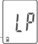
Low power (a) Action: Replace with new batteries.
